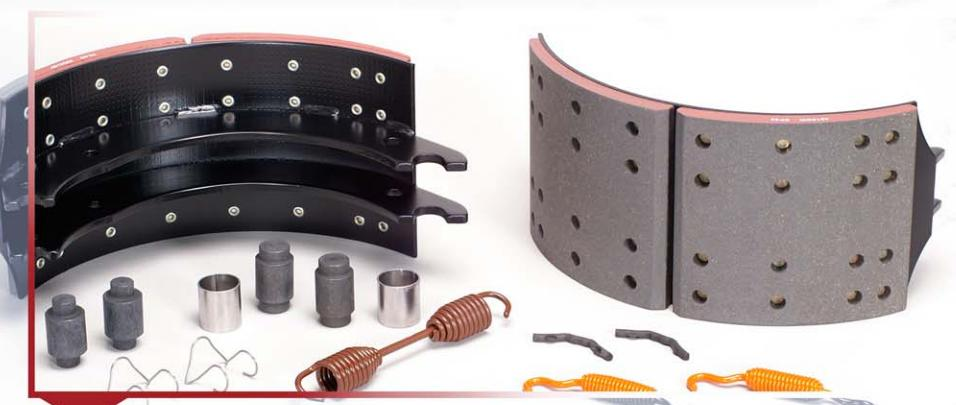
**Lined Brake Shoes and Shoeboxes.** Available with domestic brand or our imported lining in 20k, 23k or 25k ratings for all the popular steer, drive and trailer axle applications. (See back page for test data on our imported lining material.) Brake shoes are available either loose or in a shoebox which is two lined shoes with the appropriate hardware kit.
